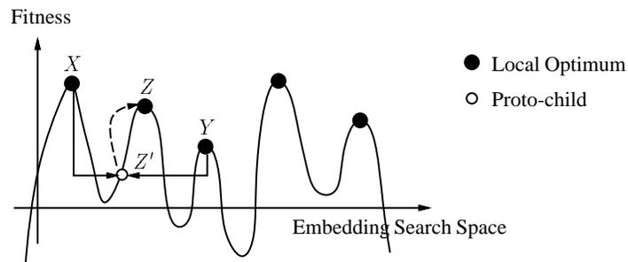
**Fig. 1.** Memetic algorithms search over the subspace of local optima within the embedding search space of all solutions. After recombination, the proto-child typically lies outside this subspace and a local optimiser is used to “repair” the child so that it lies at a local optimum. Here parents  $X$  and  $Y$  produce the proto-child  $Z'$ , which is then optimised to produce the final child  $Z$ .
