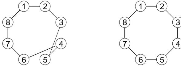
**Fig. 2.** In the undirected edge representation, the left-hand tour is  $\{1-2, 2-3, 3-5, 4-5, 4-6, 6-7, 7-8, 1-8\}$  and the right-hand tour is represented by  $\{1-2, 2-3, 3-4, 4-5, 5-6, 6-7, 7-8, 1-8\}$ . In this representation, these two tours are minimal mutations of each other, because they differ by exactly two edges and no pair of distinct tours, in this representation, differ by fewer than two edges.
