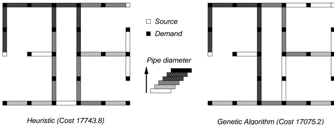
Figure 9: The genetic algorithm finds a solution approximately 4% cheaper (in cash terms) than that found by the heuristic technique and actually used for the installed network. The networks are shown only schematically: the pipes are actually of different lengths. The demand and supply requirements are also different at each node. Both networks are valid in that they satisfy both the upstream-pipe and minimum pressure constraints.
